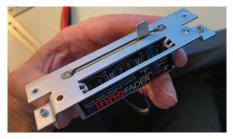
Another thing that may stump you at first is the crossfader mounting. A&H designed the plate for mounting the crossfader specifically so it can handle the 65mm hole spacing common to all Innofader models.
