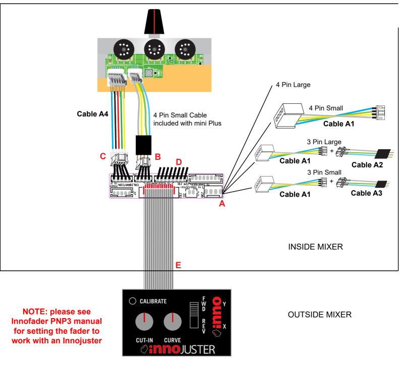
Starting with the Innofader already installed and working, please wire the Innojuster as follows:
