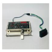
Use the mini black screws to assemble the bracket to the fader. When properly assmbled, the stem will travel freely back and forth.
