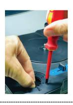
Slide the fader into the slot, and hold it at the desired angle with one hand. Make sure the outer ring of screw holes aligns with the mini Innofader Pro holes.
